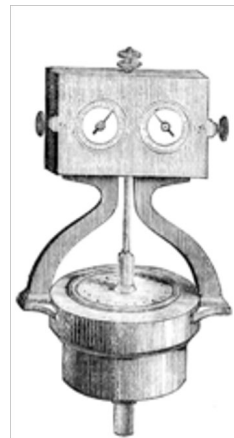
Right: Detail from an engraving of an early siren mechanism, unknown artist, Harper's New Monthly Magazine, issue 270 (November 1872); Left: Roland Zumbühl, horns in the village of Bretzwil, Switzerland, 26.10.2005 (Wikimedia)
